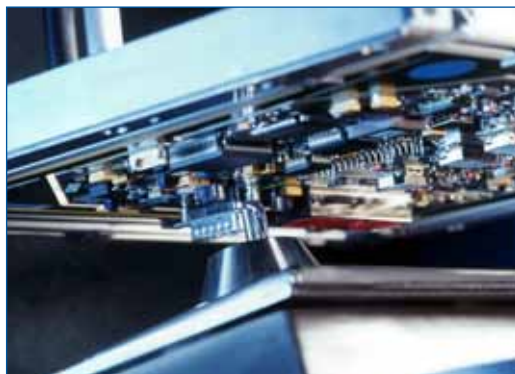
Fig 1: Soldering selective points on the underside of the board
