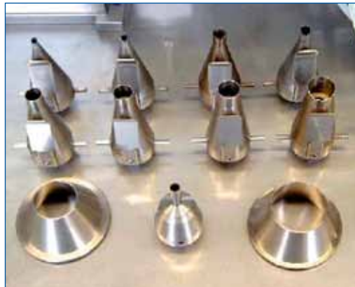
Fig 2: Some nozzle configurations that are commonly used in selective soldering applications
